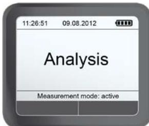
The yellow LED is flashing during the evaluation of the breath sample. Depending on the alcohol concentration this can take several seconds. Device indicates end of the analysis with a single audible signal.
