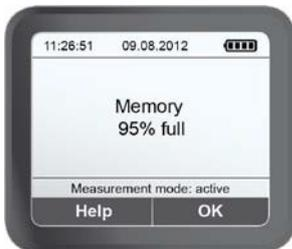
Once the internal memory is 95% full (9,499 measurements), a "Memory 95% full" message appears in the display.
