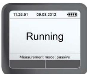
The measurement is automatically started by blowing into the device.
