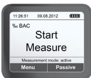
After switch-on the device operates automatically in the active mode and the Display shows "Start Measure".
